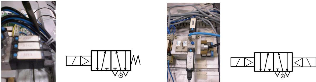
Figure 2.30 (left) single solenoid valve; (right) double solenoid valve
