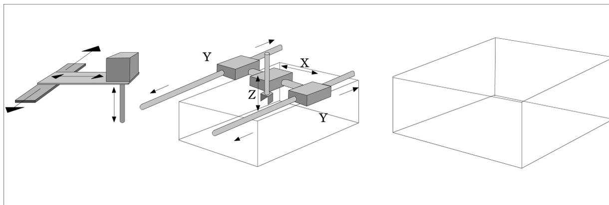
Figure 4.4 Schematics diagram of Cartesian robots
