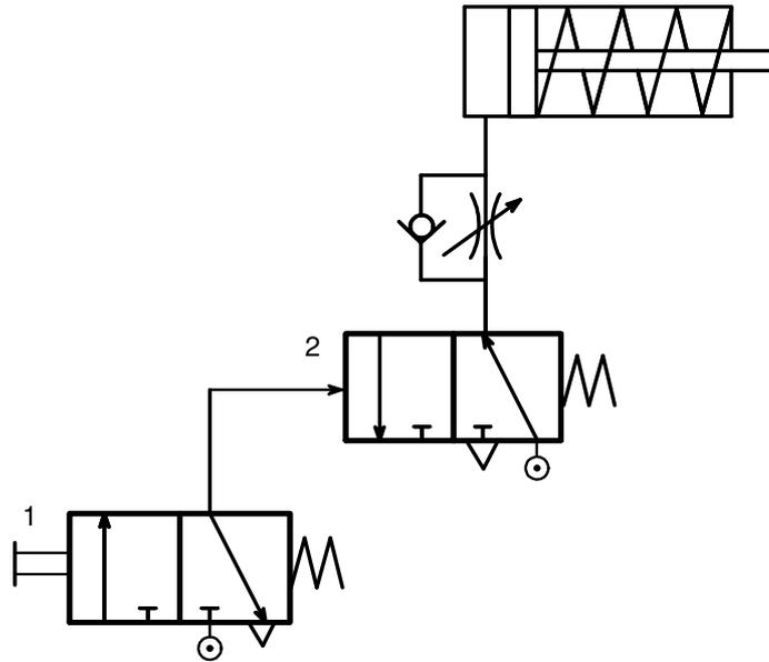
Figure 2.23 Signal inversion of a cylinder
