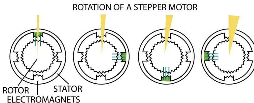
Figure 3.31 Alternate energizing stator for the rotation of rotor.
