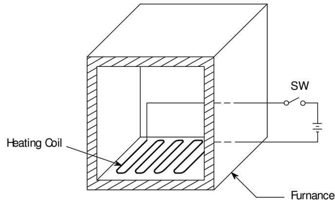
Figure 1.2 Open-Loop control system of Furnace Temperature (Controlled value)
