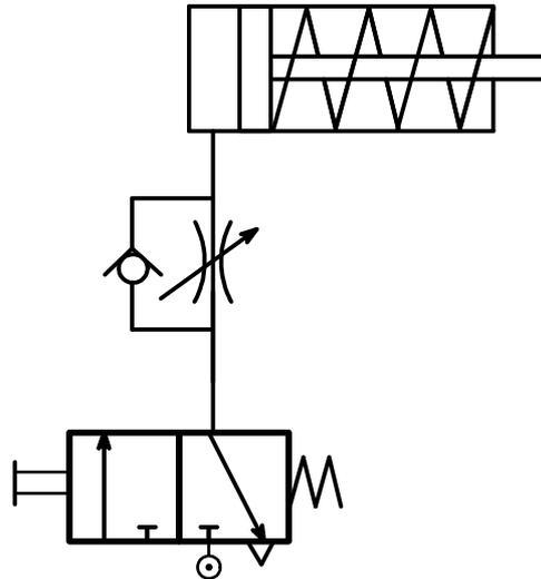
Figure 2.20 Direct control of a single acting cylinder
