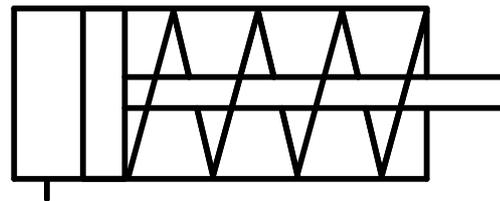
Figure 2.10 Structure and symbol of Single acting cylinder
