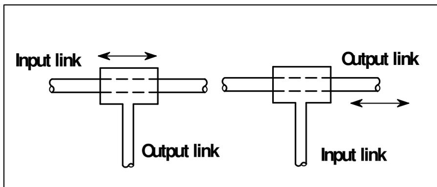
Figure 4.19 Two types of orthogonal joint are also known as Type O
