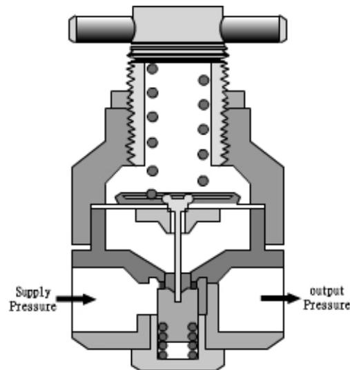
Figure 2.4 Regulator sectional diagram
