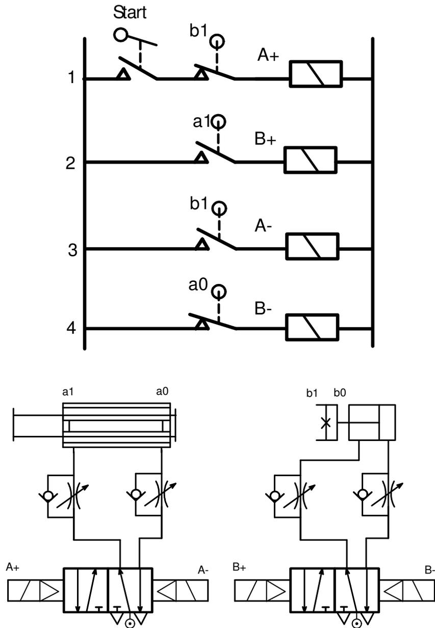
Figure 2.43 Sequential controls of pneumatic slide and gripper
