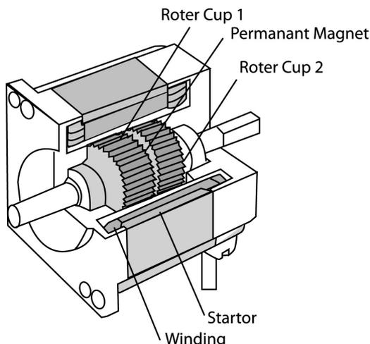
Figure 3.30 Exploded view of a typical stepping motor
