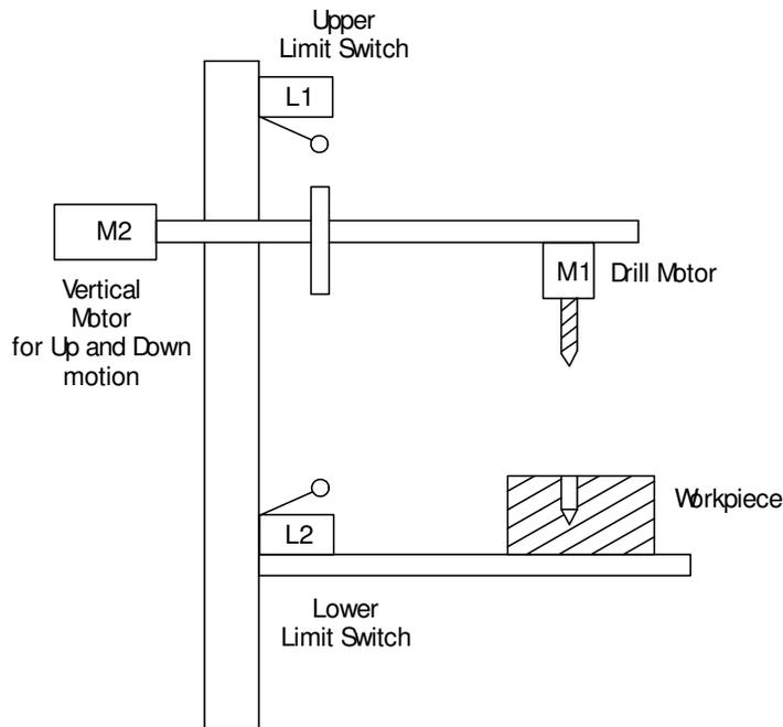
Figure 3.13 Schematic diagram of automatic drilling system
