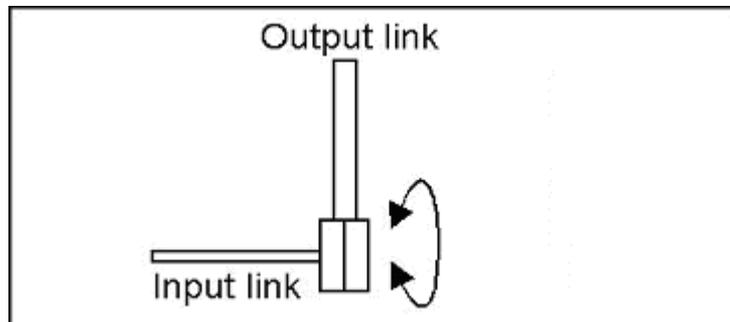
Figure 4.22 Output link is perpendicular to the input joint, but parallel to the axis of rotation – Type V
