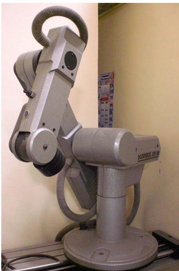
Figure 4.1 Typical industrial robotic arm.
