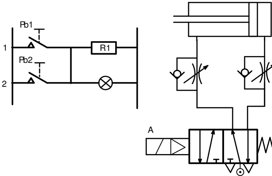
Figure 2.33 Control of cylinder and lamp by either pb1 or pb2
