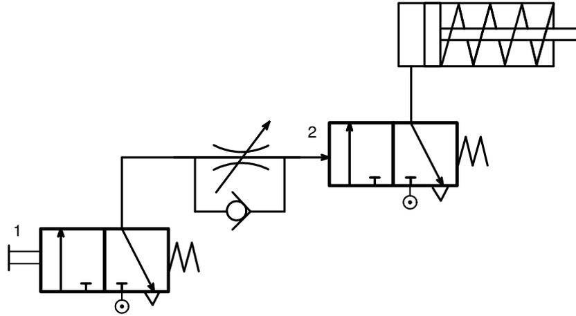
Figure 2.18 Delayed switching ON circuit
