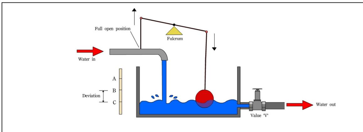
Figure 1.21 Valve fully open
