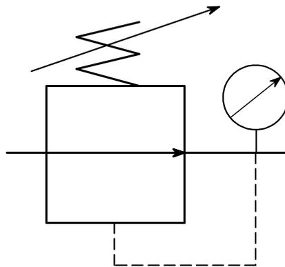
Figure 2.5 Structure and symbol of a Pressure Regulator
