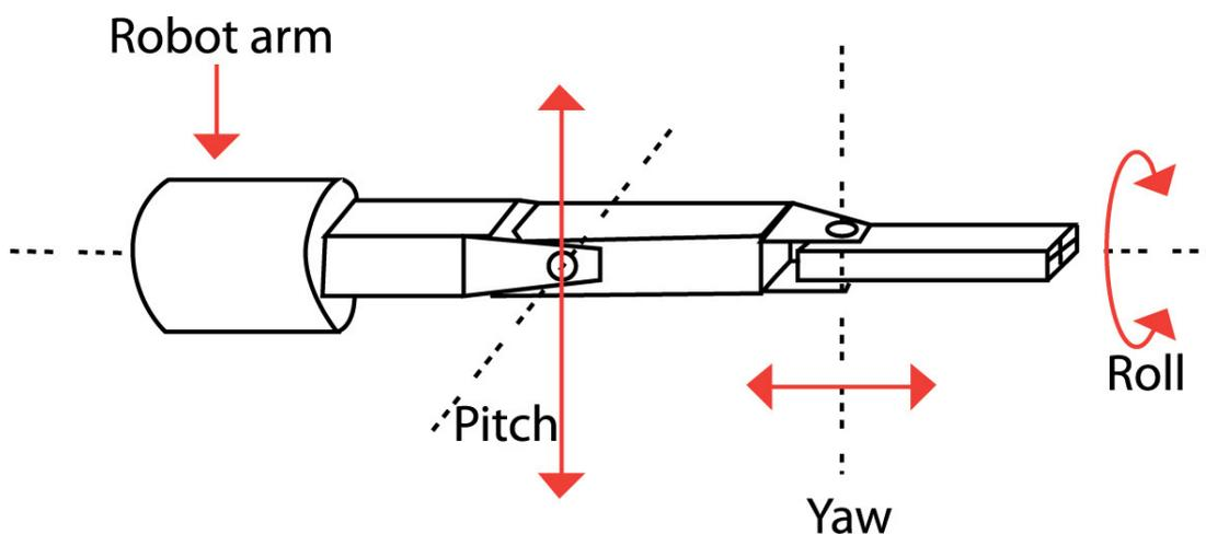
Figure 4.17 A typical wrist would have 3 DOF
