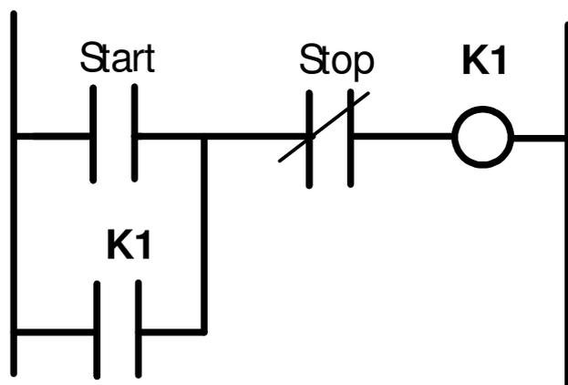
Figure 3.8 Ladder diagram of motor ON/OFF control
