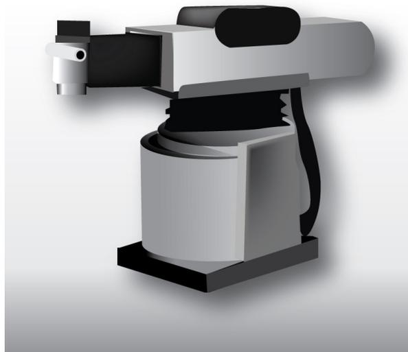
Figure 4.5 Typical Cylindrical Robot
