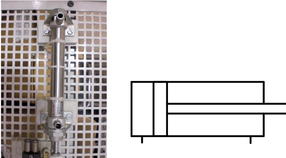
Figure 2.11 Structure and symbol of Double acting cylinder
