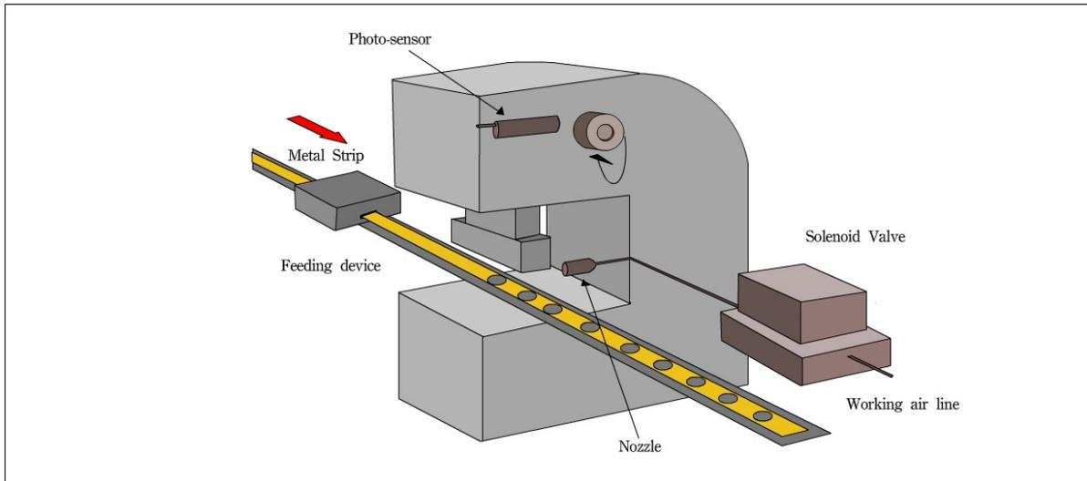
Figure 2.60 Punching Machine Accessory Function
