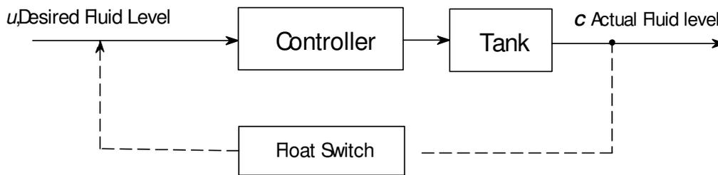
Figure 1.18 Block diagram of fluid level control system
