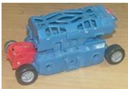
Figure 4.2 Toys chassis used as a locomotive platform
