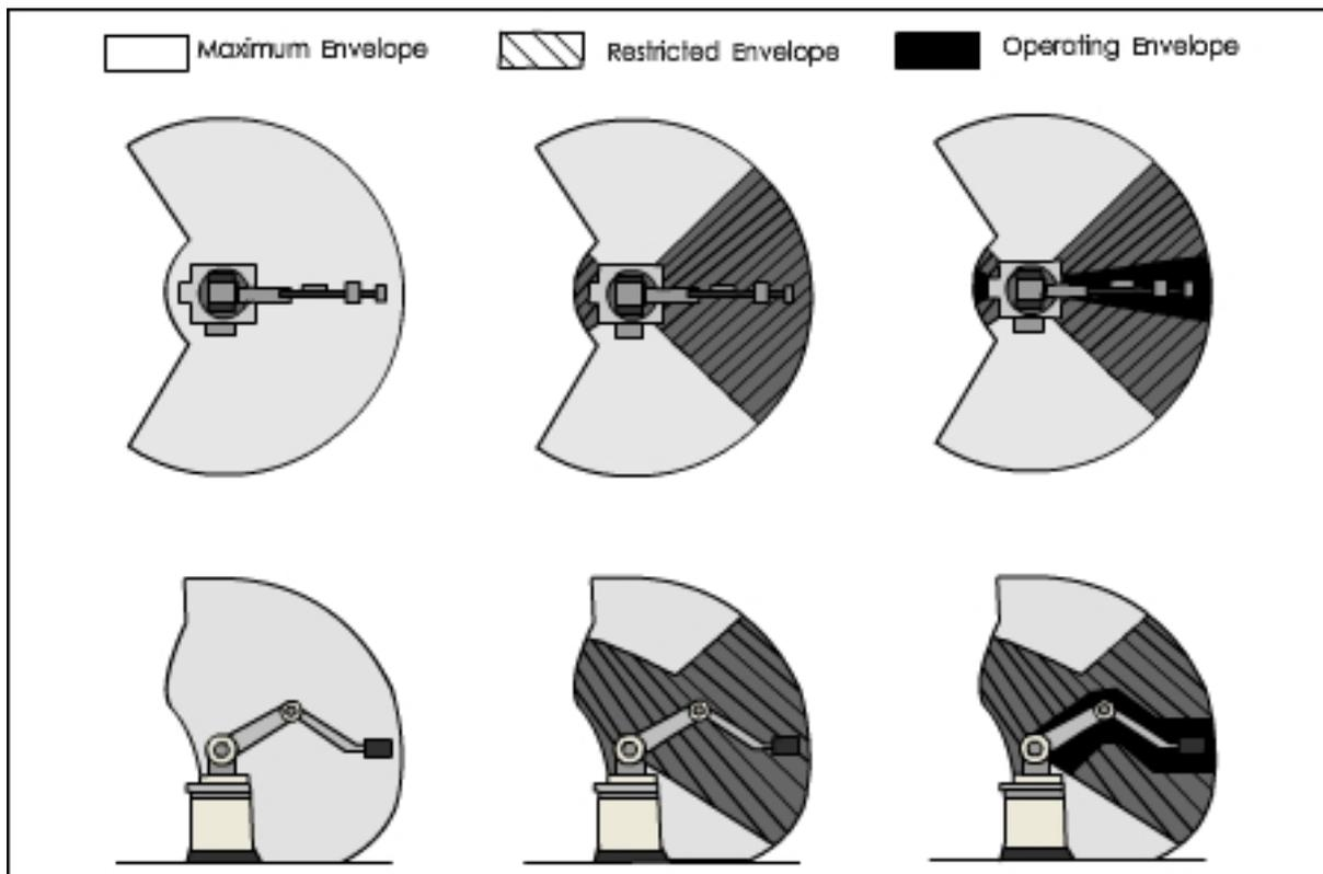
Figure 4.28 Diagrams show the work envelopes of an articulated robot
