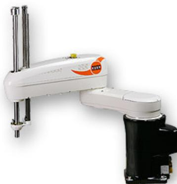
Figure 4.9 Typical SCARA Robot
