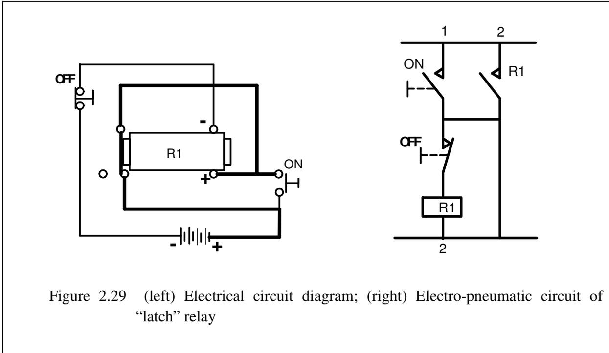
Figure 2.29 (left) Electrical circuit diagram; (right) Electro-pneumatic circuit of “latch” relay
