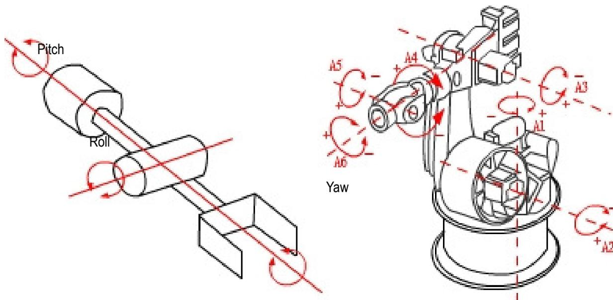
Figure 4.14 Schematic diagram of Articulated Robots
