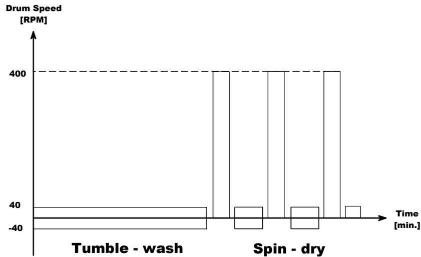
Figure 1.9 Timing diagram for washing processes
