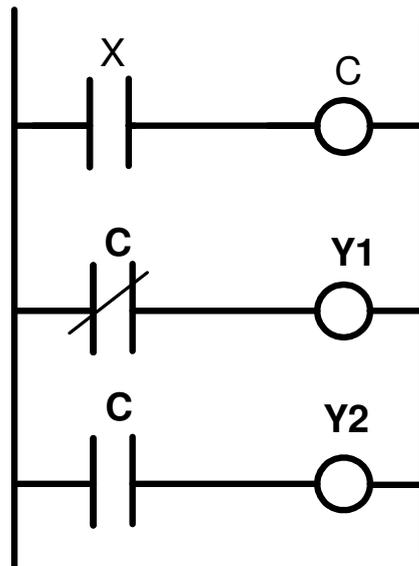
Figure 3.10 Use of control relay for multiple logic function
