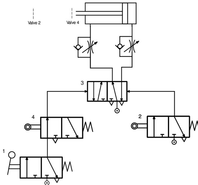
Figure 2.27 Reciprocating stroke of a double acting cylinder
