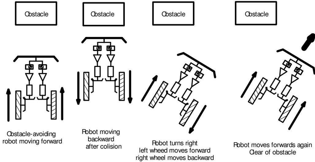
Figure 1.24 The basic operation of the obstacle-avoiding buggy
