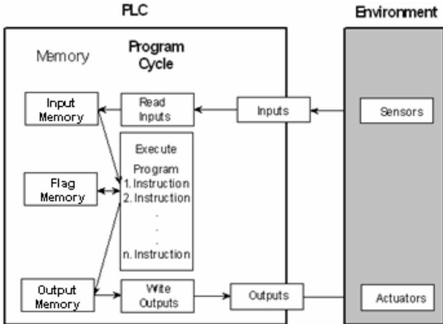
Figure 3.3 Functionality of PLC components
