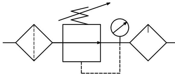
Figure 2.6a Structure and symbol of a combined APU
