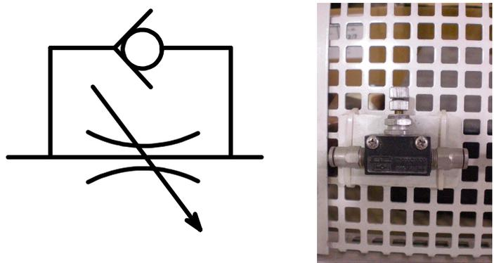
Figure 2.8 Structure and symbol of flow control Valve
