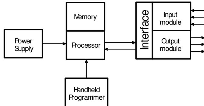
Figure 3.2 Schematic diagram of the basic Programmable Logic Controller
