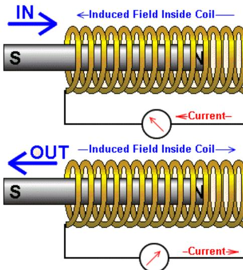
Figure 4.31 Operation of solenoid actuator
