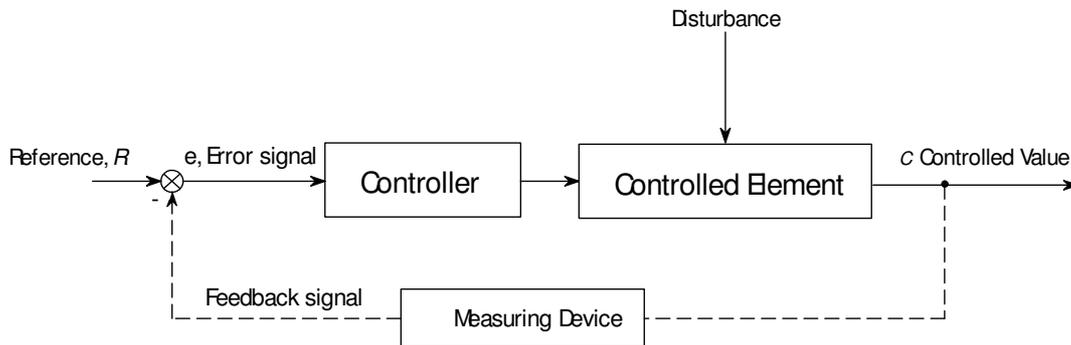
Figure 1.6 Block diagram of Closed-Loop control system
