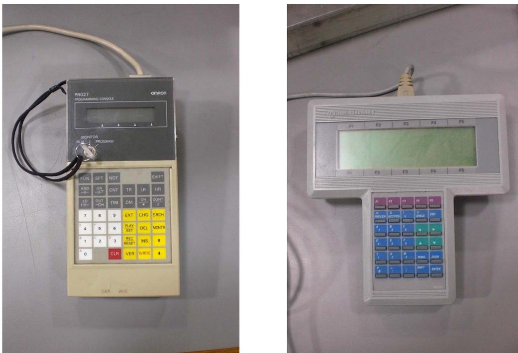
Figure 3.16 Handheld Programmer for PLCs
