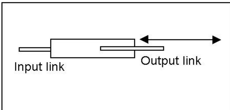
Figure 4.18 Radial, sliding, or translational movement – Type L
