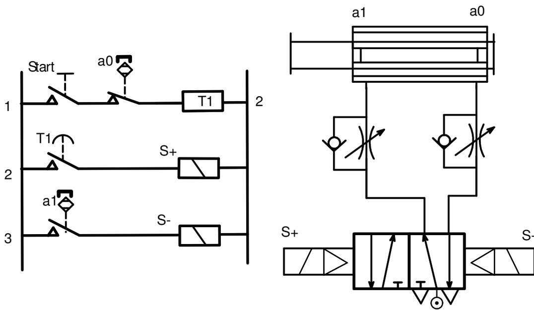
Figure 2.40 Double acting cylinder with delay on timer in extend stroke
