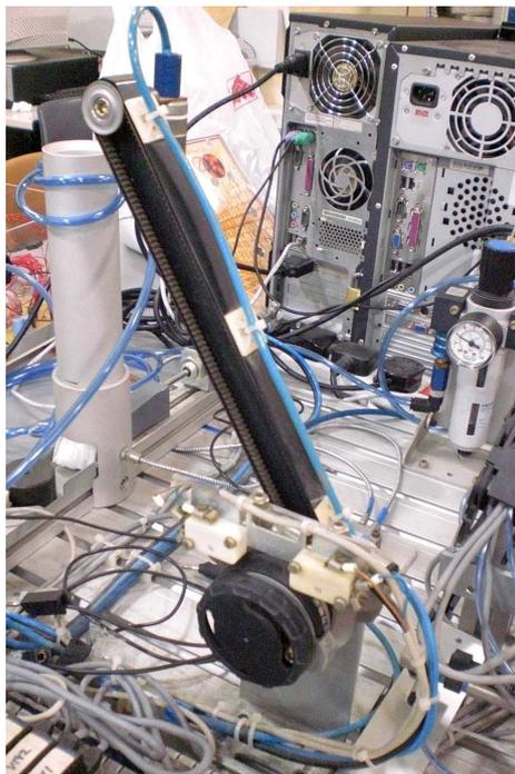
Figure 2.38 Rotary Actuator
