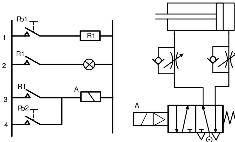
Figure 2.34 Control of cylinder and lamp by pb1; pb2 for controlling cylinder only.
