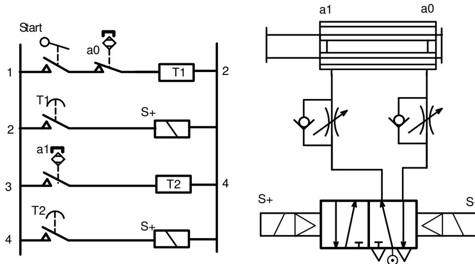
Figure 2.41 Double acting cylinder with delay-on timer in both extend and retract stroke
