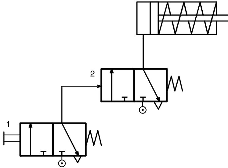
Figure 2.14 Flow amplification and remote control of cylinder
