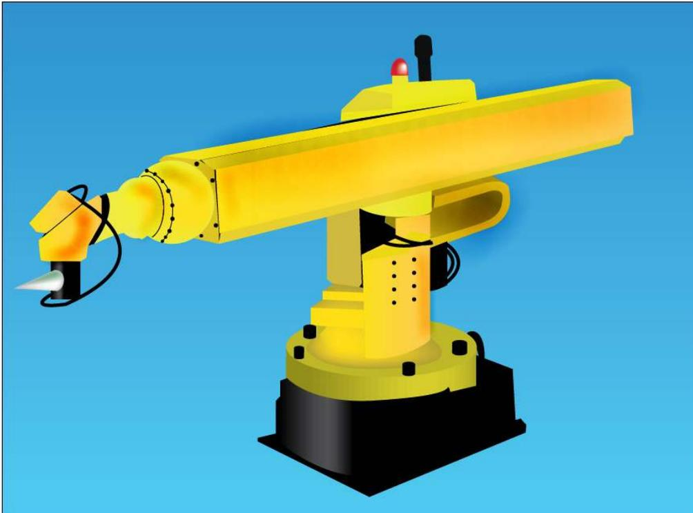
Figure 4.7 Typical Polar Robot
