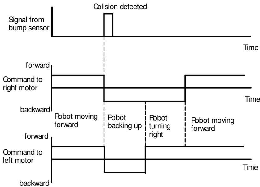
Figure 1.25 Timing sequence illustrating the obstacle-avoiding buggy's backing up behavior.
