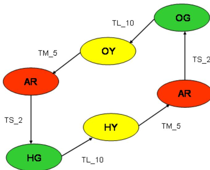
Figure 2.2 State diagram for the traffic lights intersection
