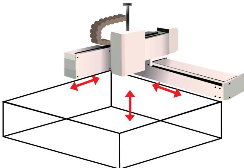
Figure 4.3 Typical Cartesian Robot
