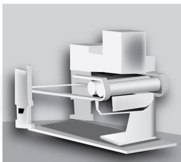
Figure 4.41 Construction Robot for pavement work
