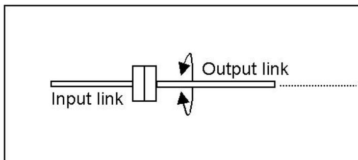
Figure 4.21 Axis of rotation is parallel to the links – Type T
