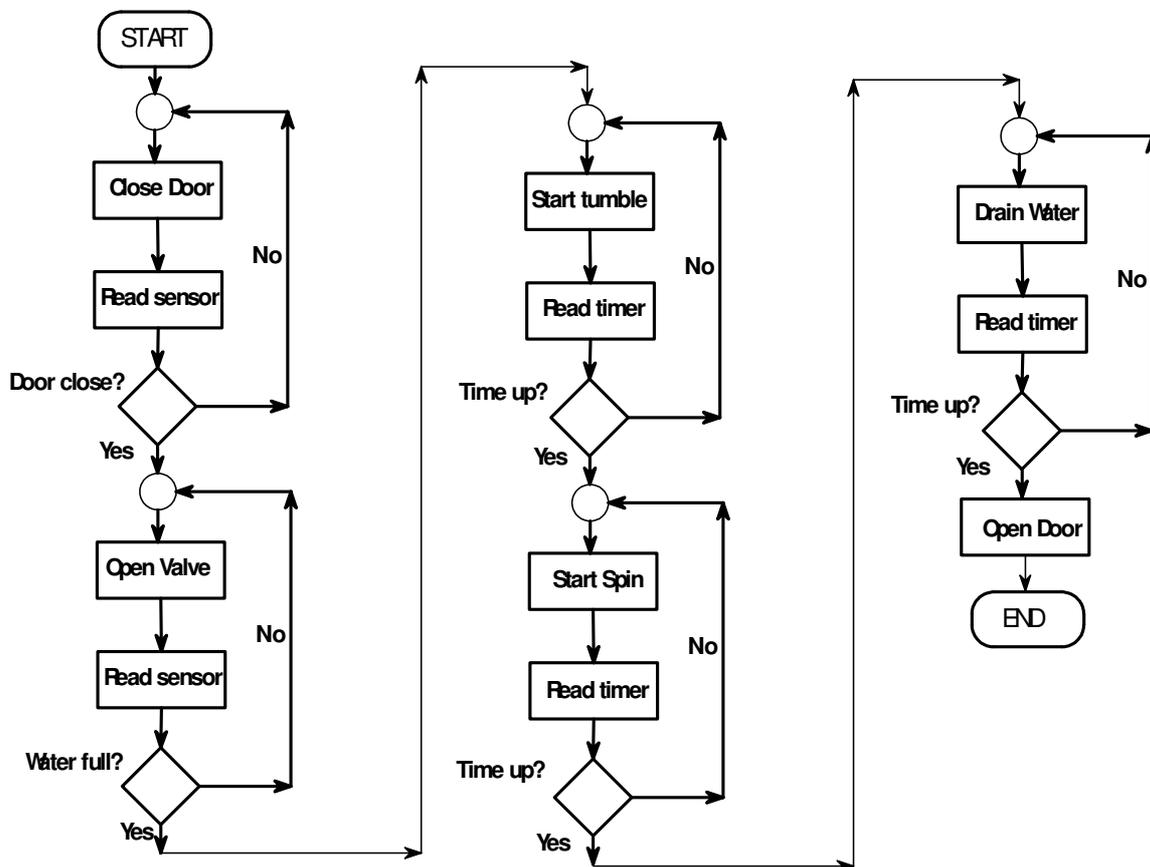
Figure 1.11 Flow diagram for a classical washing machine
