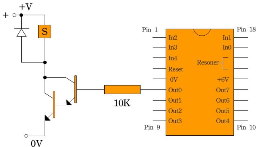
Figure 3.27 Output circuitry for Solenoid
