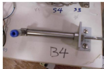
Figure 4.32 Pneumatic cylinder
