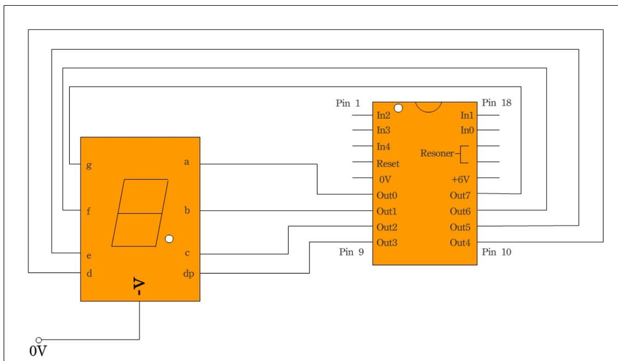
Figure 3.23 Output circuitry for 7 segment display
