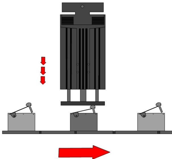
Figure 2.45 Testing of limit switches
