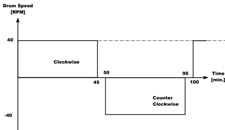
Figure 1.10 The timing phase diagram for tumble-wash phase
