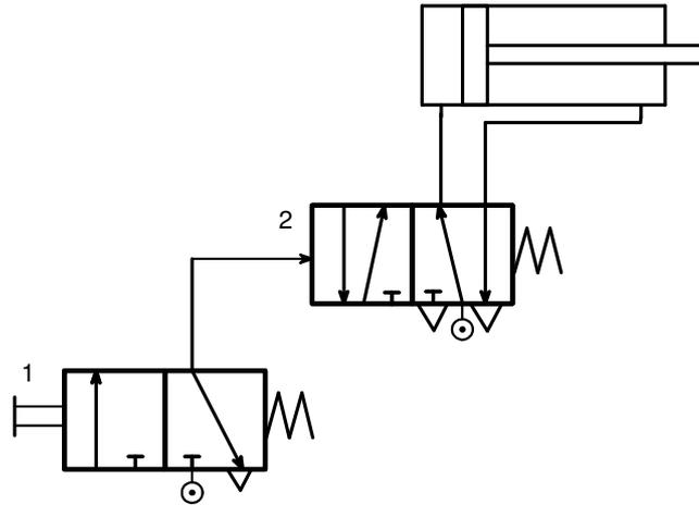
Figure 2.16 Switching of two circuits with one manual operated valve
