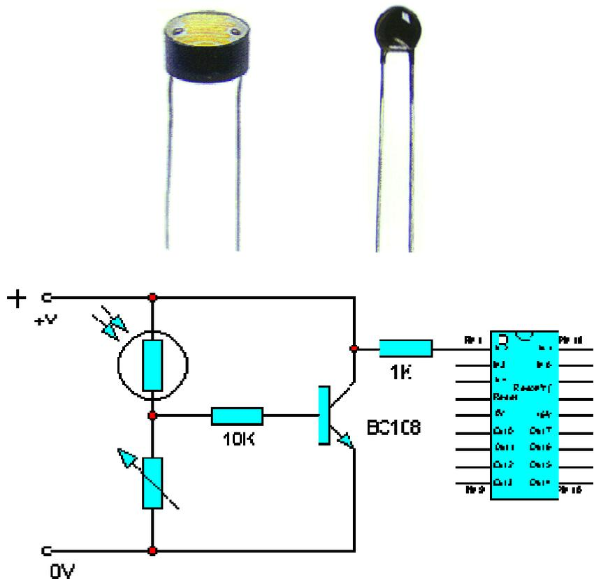
Figure 3.20 Interfacing circuit for analogue photo-sensors
