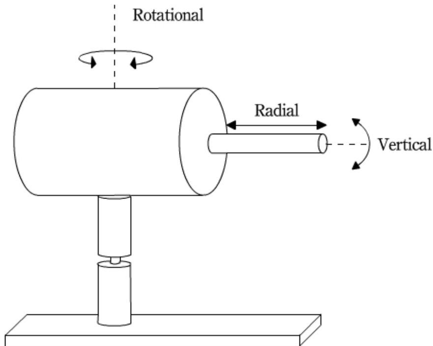
Figure 4.16 Combination of vertical, radial and translational movements
