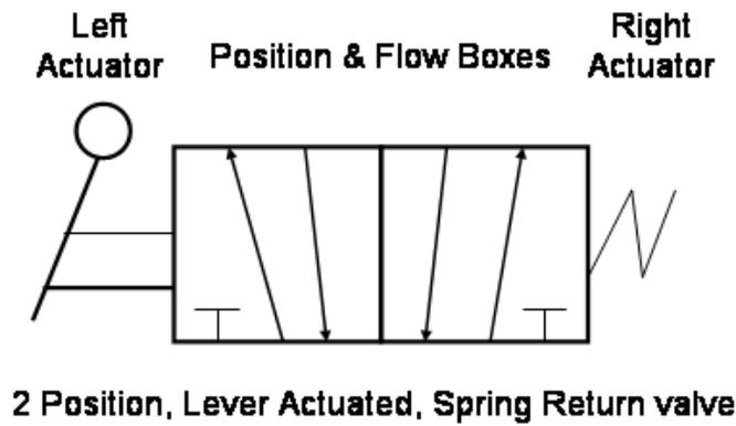
Figure 2.7 Directional Valve symbol
