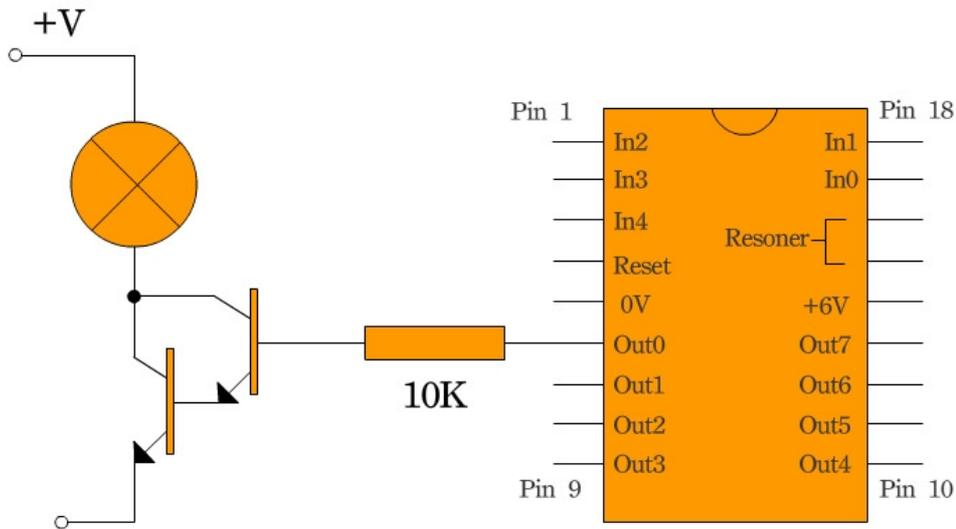
Figure 3.26 Output circuitry for Light bulb
