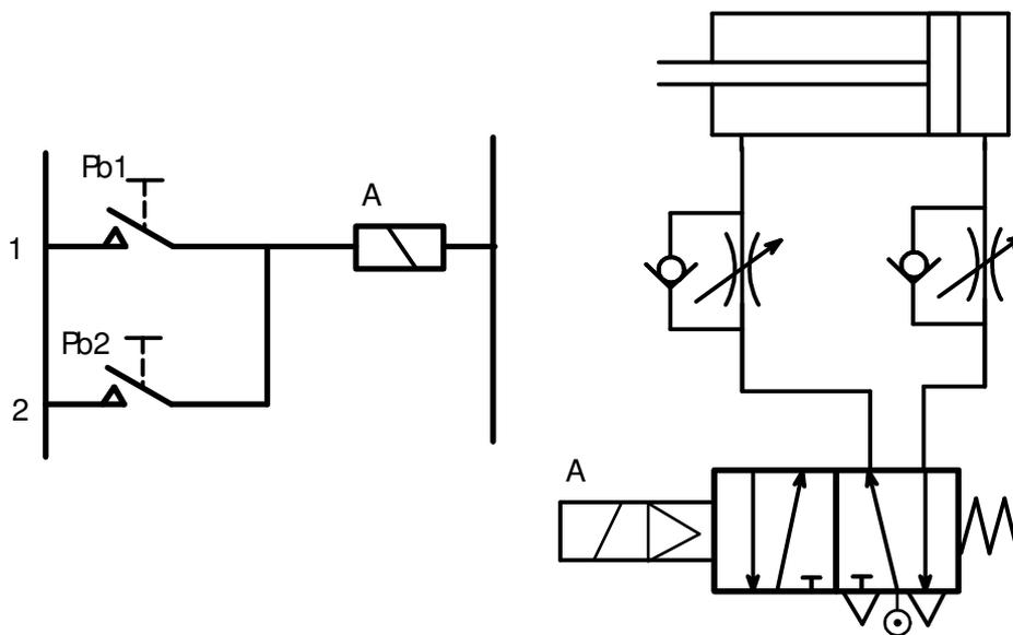
Figure 2.32 “OR” operation of double-acting cylinders
