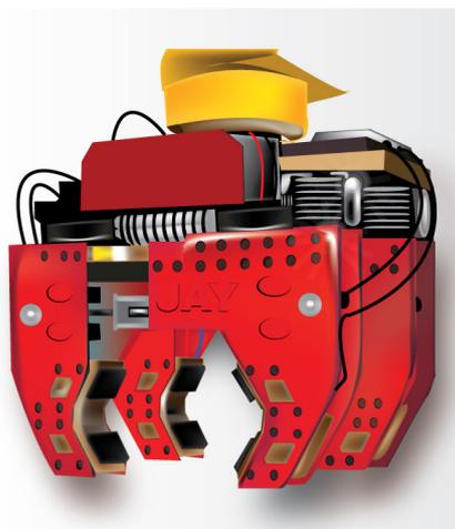
Figure 4.26 Mechanical gripper of fingers type
