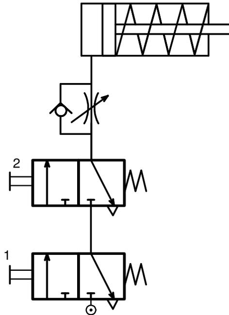
Figure 2.22 Interlock and “AND” function of a single-acting cylinder
