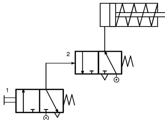
Figure 2.15 Circuit diagram of Signal inversion
