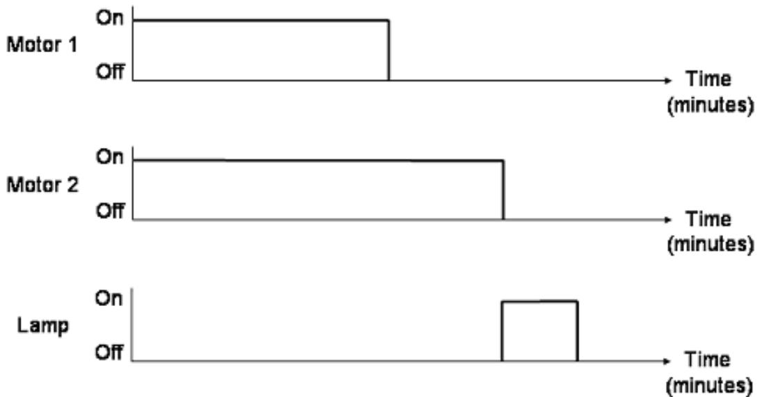
Figure A.9 Timing diagram for the operation sequence
