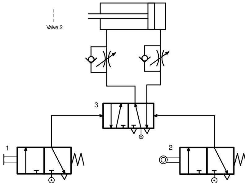
Figure 2.26 Automatic control of a double acting cylinder
