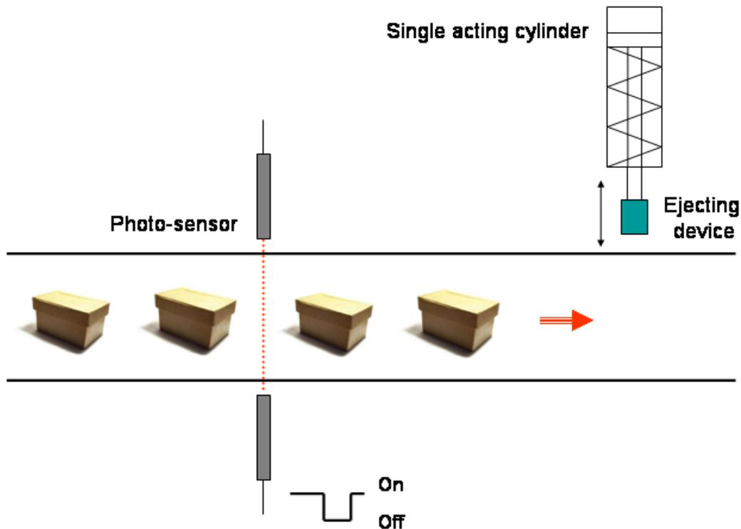
Figure A.10 Schematic diagram of the system
