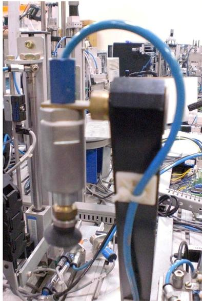
Figure 4.24 Vacuum gripper
