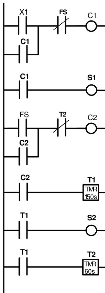
Figure 3.12 Ladder logic diagram for fluid level control
