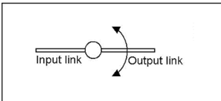
Figure 4.12 Axis of rotation is perpendicular to axis of the 2 connecting links – Type R
