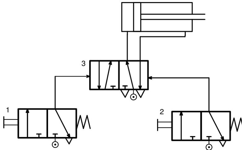
Figure 2.17 Switching of two circuits with one manual operated valve
