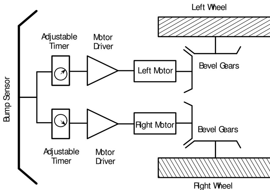
Figure 1.23 The block diagram shows two motors, two wheels, a bump sensor and two potentiometers for programming the time events.
