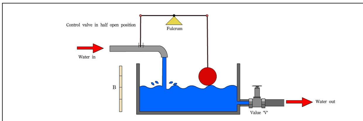
Figure 1.19 Valve at 50% open
