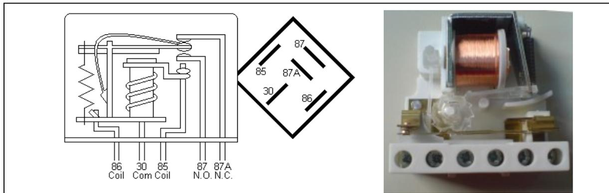
Figure 2.28 Schematic diagram of electro-mechanical relay principle.
