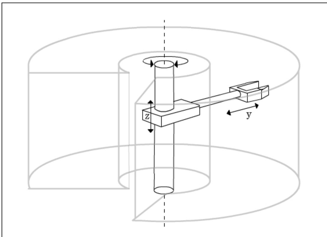
Figure 4.6 Schematics diagram of Cylindrical Robot
