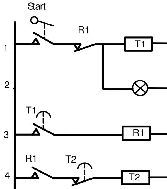
Figure 2.42 Control of bi-stable LED flashing
