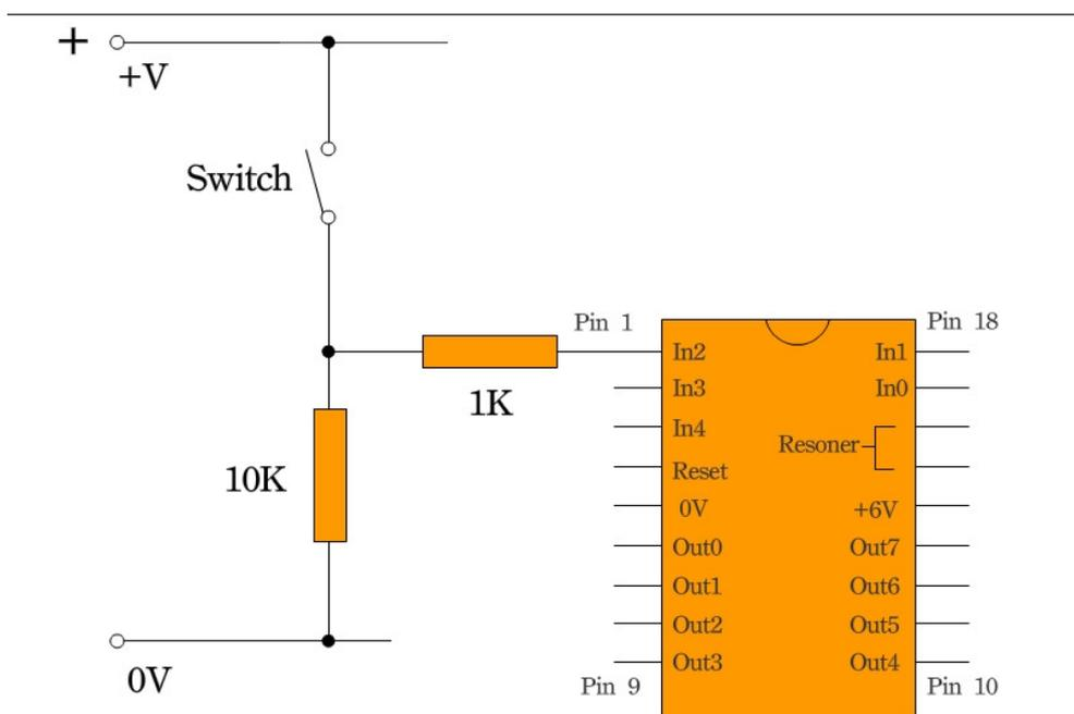
Figure 3.19 Circuit diagram for connecting input device
