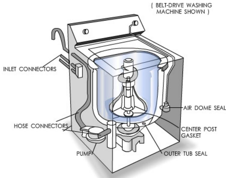
Figure A.1 A cutaway view of a washing machine
