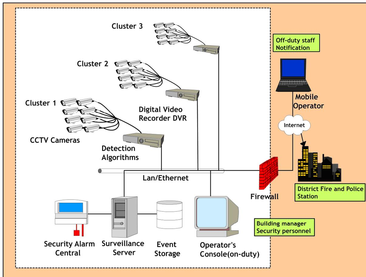
Figure 1.3 Block diagram of Intelligent Fire Alarm system
