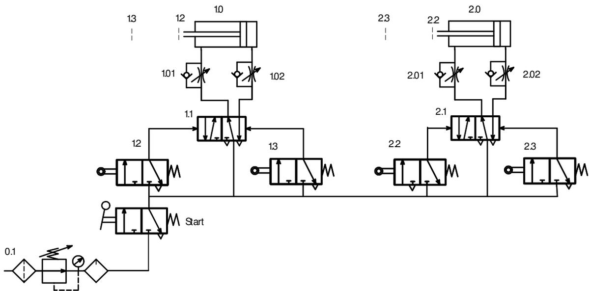
Figure 2.13 Pneumatic circuit with number notation
