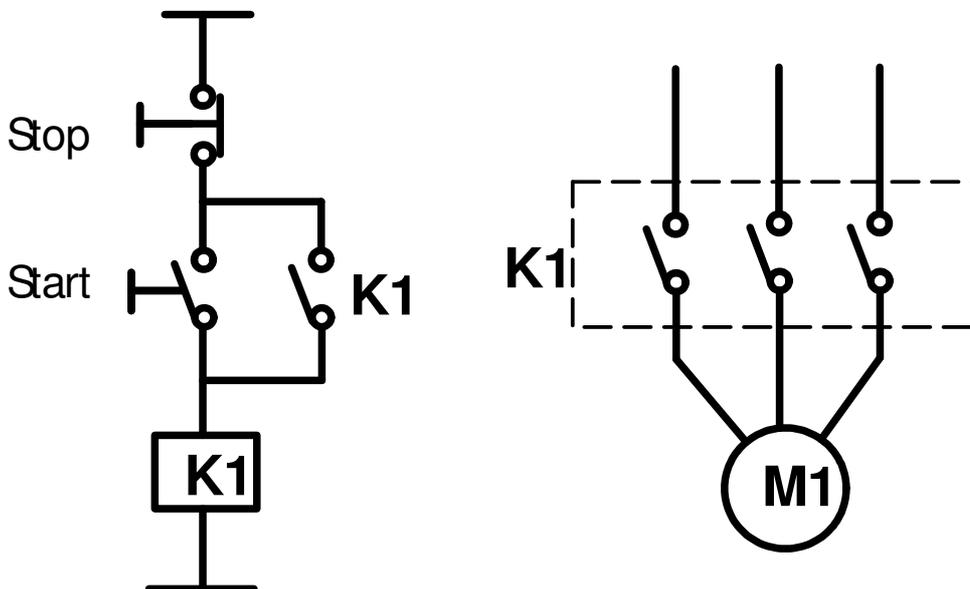
Figure 3.7 Motor ON/OFF control (Industrial 3 phase motor)
