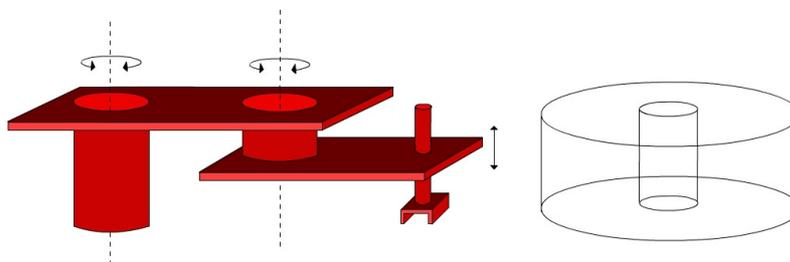
Figure 4.10 Work space of polar robot
