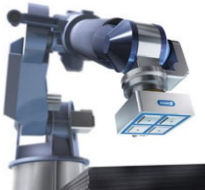
Figure 4.25 Articulated robot per permanent magnetic gripper
