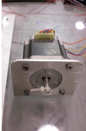
Figure 3.28 Photo of a typical stepping motor
