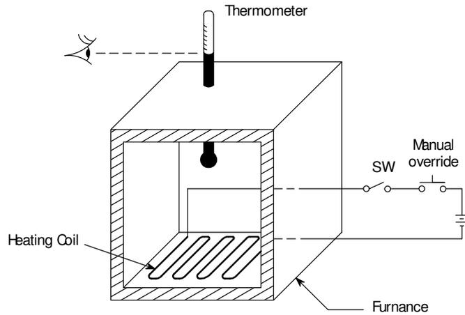
Figure 1.3 Human interrupt control of the Open-Loop control system
