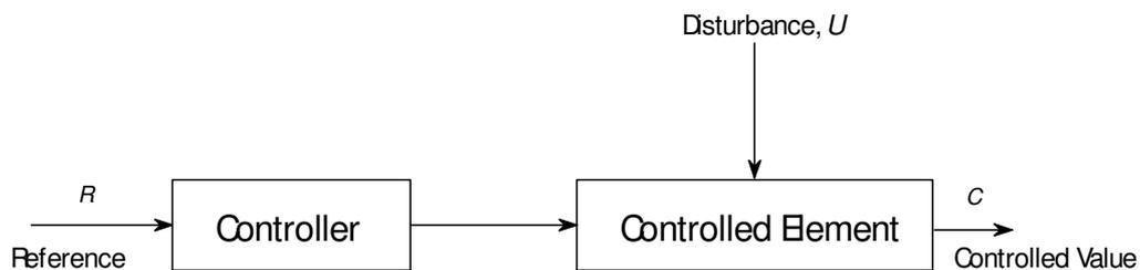
Figure 1.1 Block diagram of Open-Loop control system
