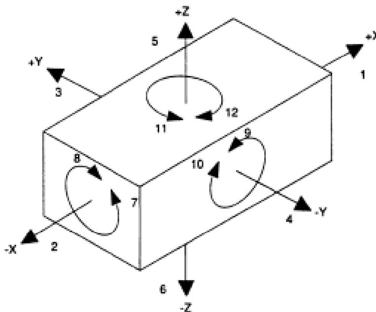
Figure 4.15 Total 12 Degree of Freedom of an object
