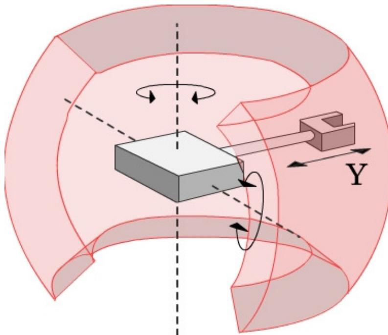
Figure 4.8 Schematics diagram of Polar robot
