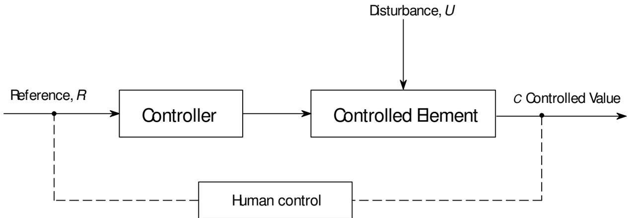
Figure 1.4 Block diagram of Human override in Open-Loop control system
