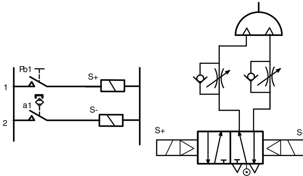
Figure 2.37 Automatic return of rotary actuator
