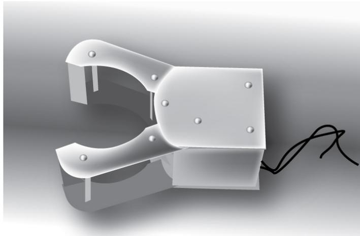
Figure 4.3 Typical 2-fingers gripper design based on linkage and driven by electric motor
