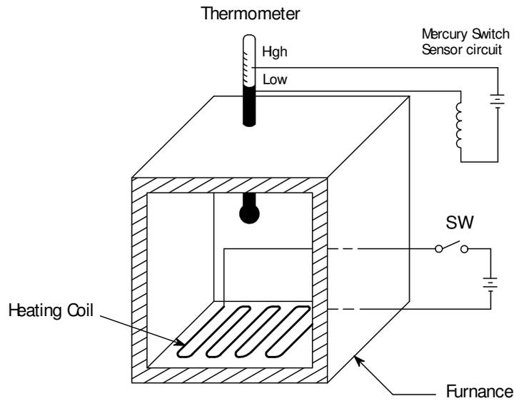
Figure 1.5 Closed-Loop control system of furnace
