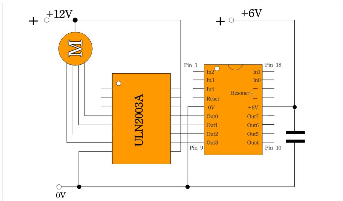
Figure 3.32 Control circuitry for stepping motor by PIC 16F84
