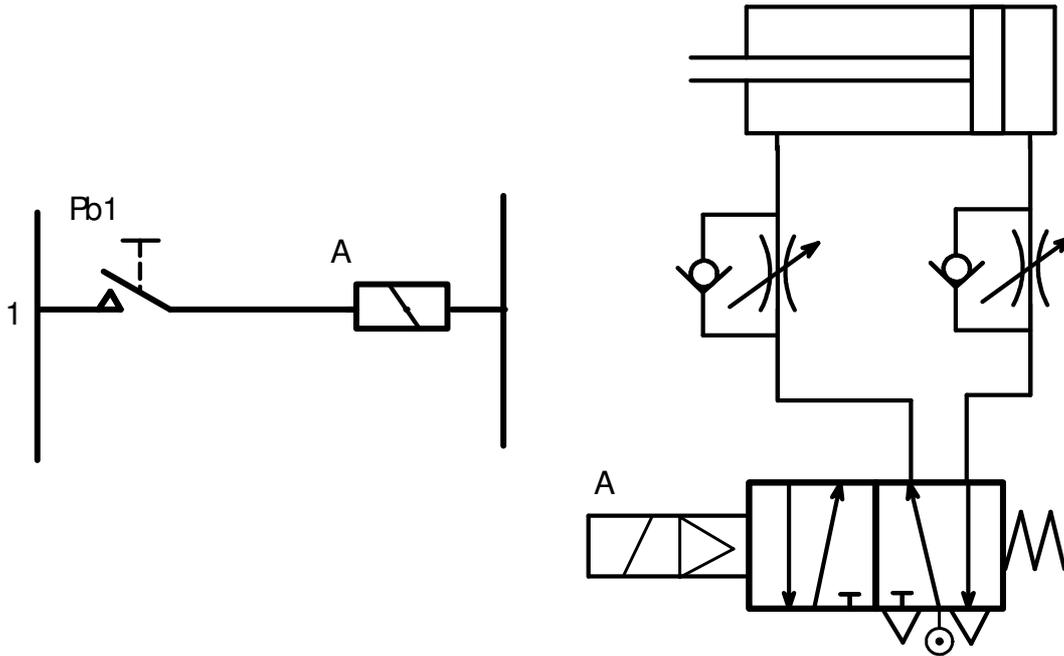
Figure 2.31 Manual operation of a double-acting cylinders
