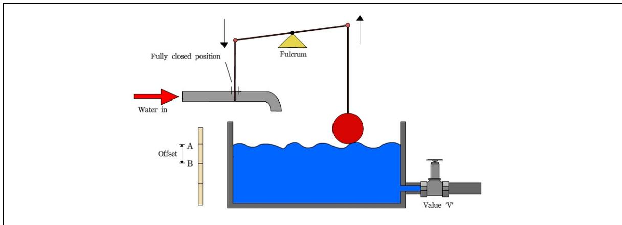
Figure 1.20 Valve fully closed
