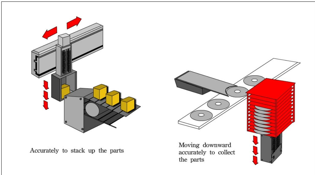
Figure 2.44 Examples of material transfer application
