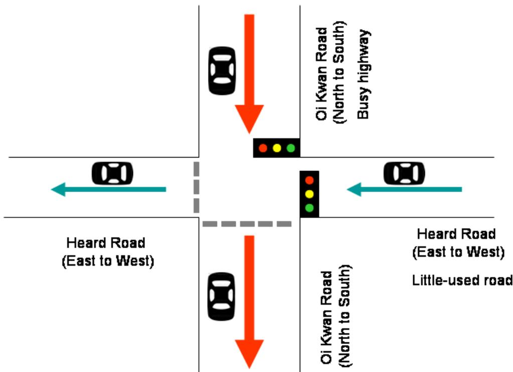
Figure 2.1 Traffic light control between Oi Kwan Road and Heard Road
