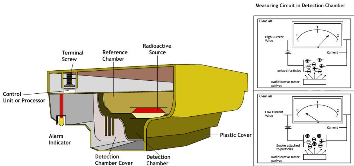
Figure 1.5 A cutaway diagram of intelligent smoke sensor
