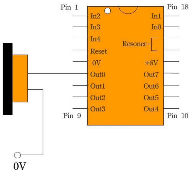
Figure 3.24 Output circuitry for Piezo speaker
