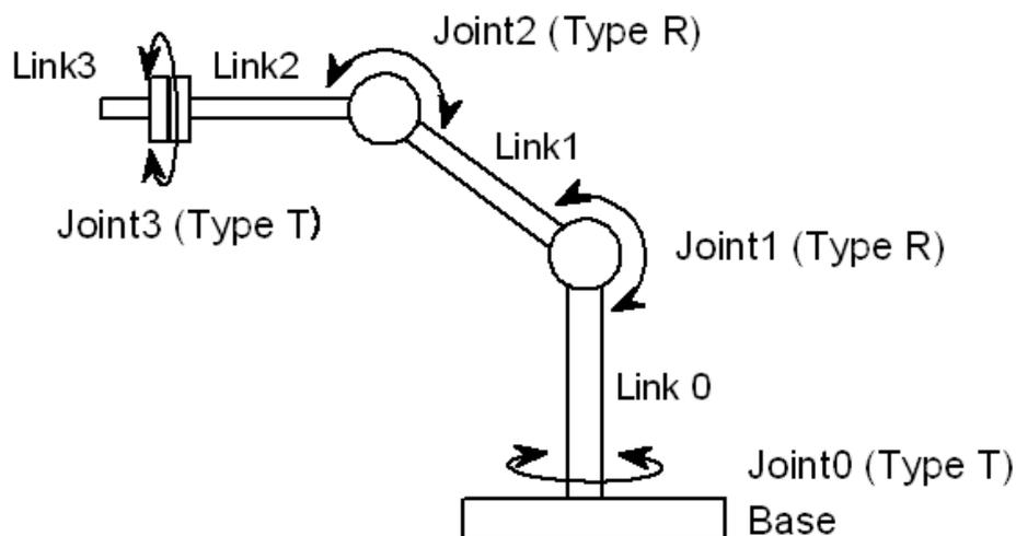
Figure 4.23 Joint and link nomination in an Articulated robot
