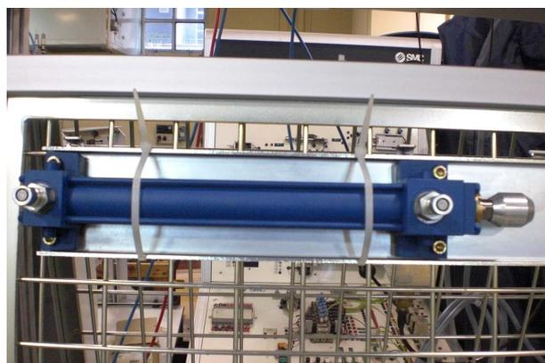
Figure 4.33 Hydraulic actuator
