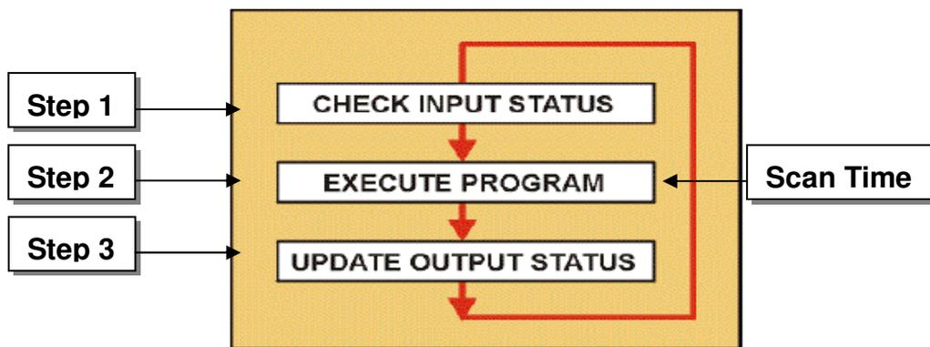
Figure 3.4 Scan cycle of PLC
