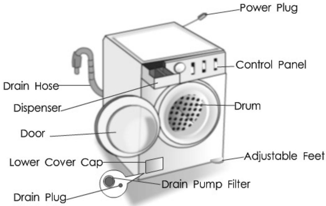
Figure 1.8 Typical structure of a washing machine
