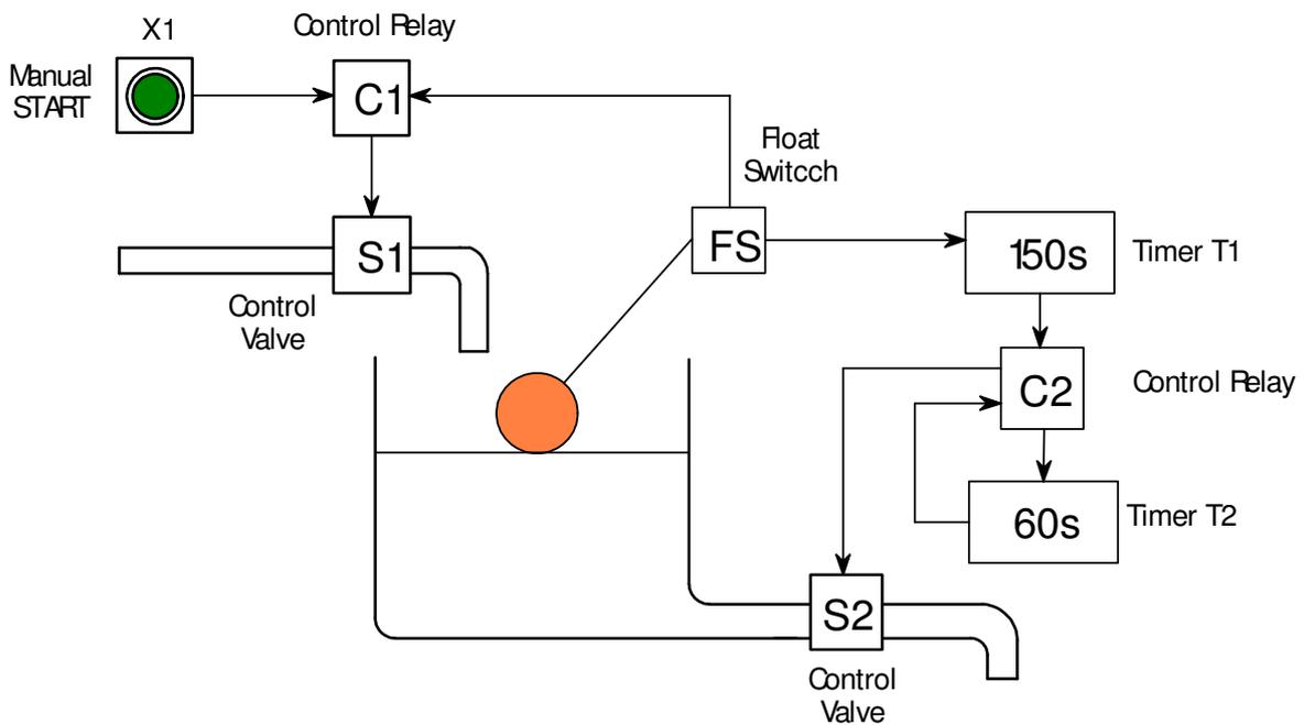
Figure 3.11 Schematic diagram of fluid level control
