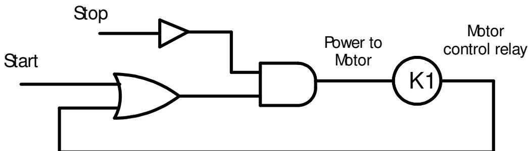
Figure 3.9 Hard-wired logic circuit for the same motor ON/OFF control
