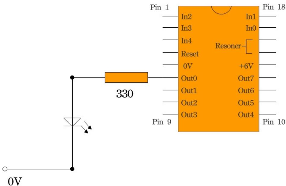
Figure 3.22 Output circuitry for LED
