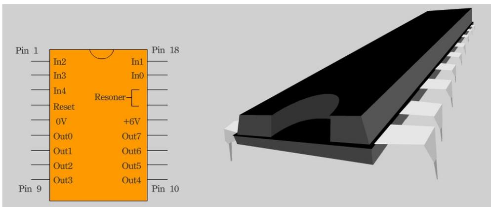
Figure 3.17 Pin layout diagram of PIC 16F84
