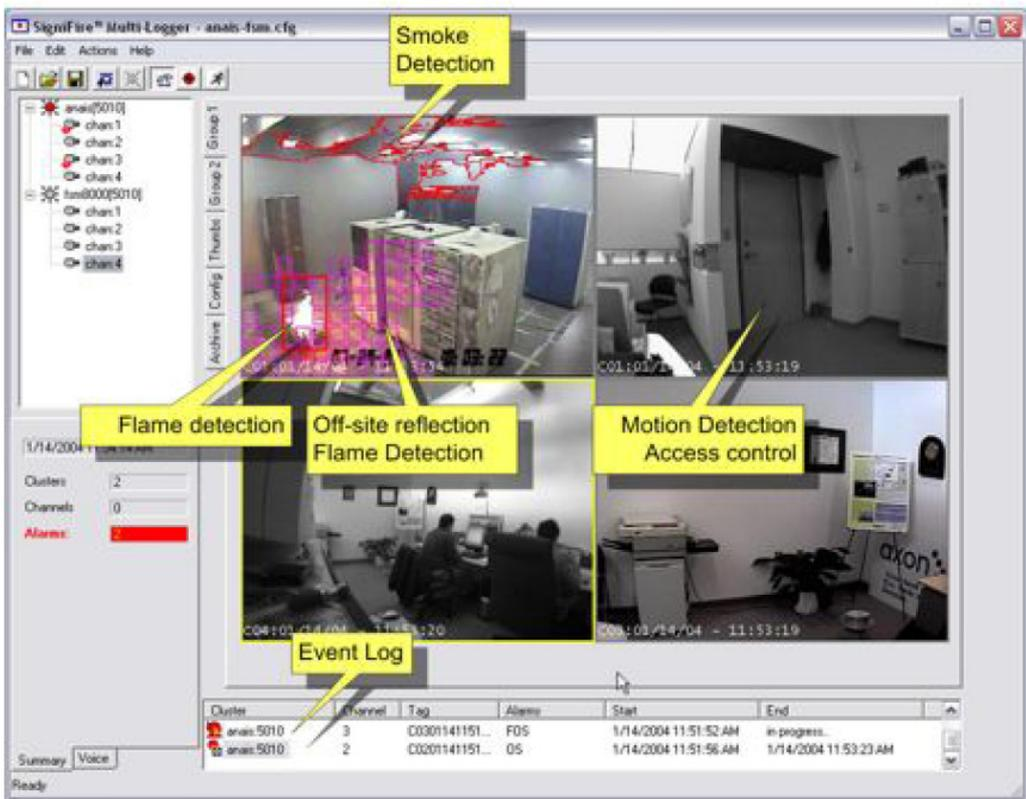
Figure 1.4 User Interface of Flame and Smoke detection system
