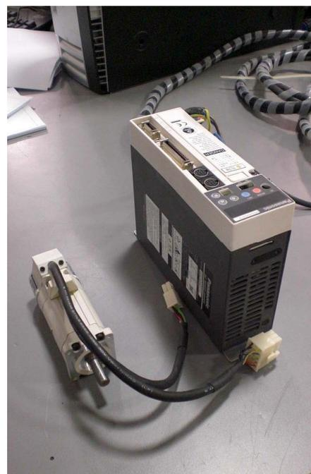
Figure 4.30 AC Servos with controller
