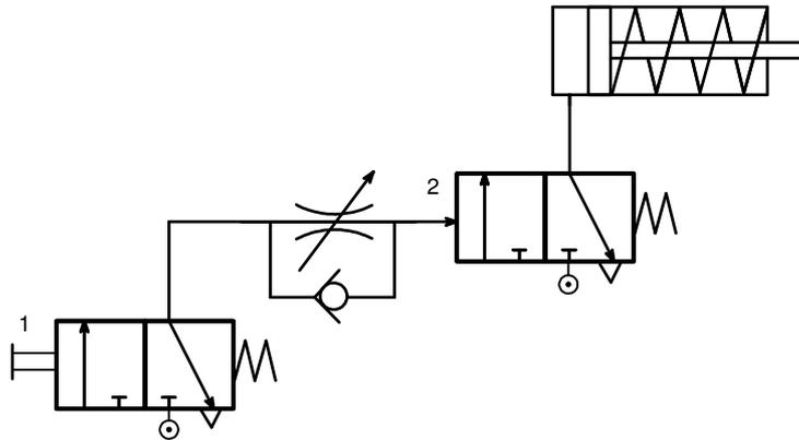
Figure 2.19 Delayed switching OFF circuit
