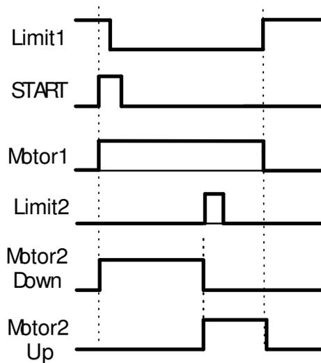
Figure 3.14 Timing diagram for sequential control of automatic drilling system
