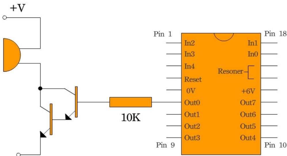
Figure 3.25 Output circuitry for buzzer
