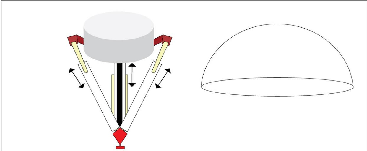
Figure 4.12 Schematics diagram of Parallel Robot
