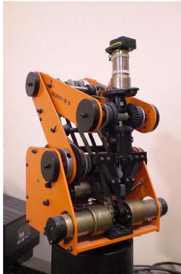
Figure 4.13 Typical **Articulated Robots** for material handling application
