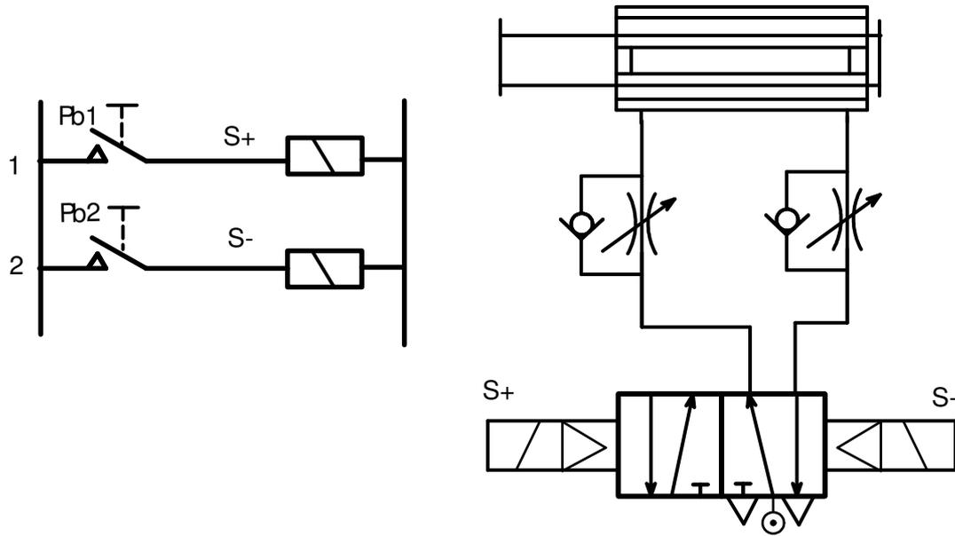
Figure 2.35 Control of Slide unit movement.
