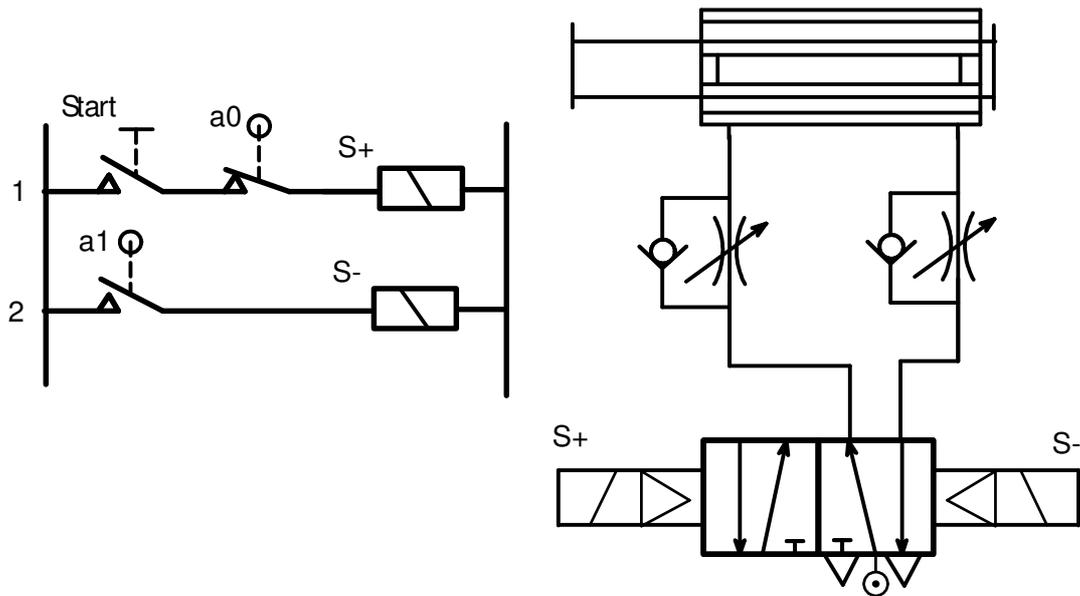
Figure 2.39 Reciprocating movement of Linear drive
