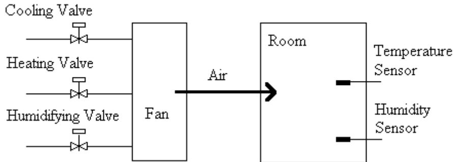
Figure 1.27 Block diagram of temperature and humidity control system
