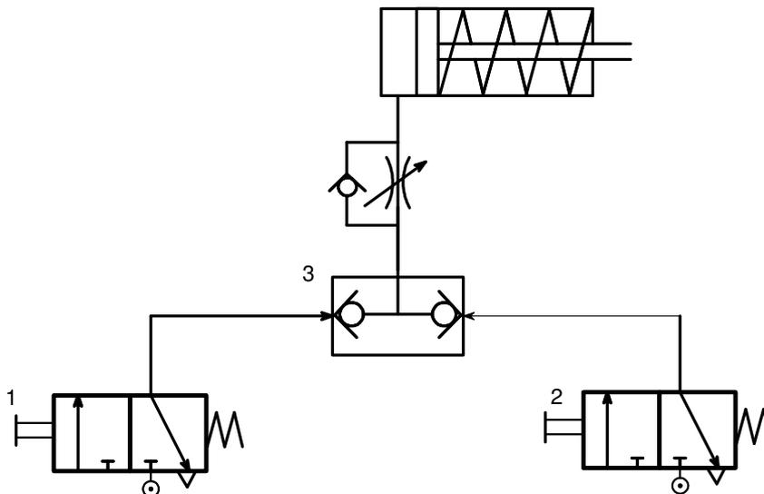
Figure 2.21 “OR” Operation of a single-acting cylinder
