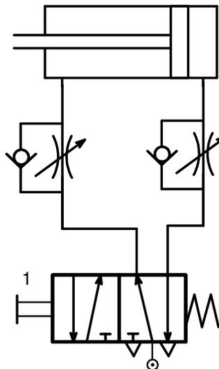
Figure 2.24 Direct control of a double acting cylinder
