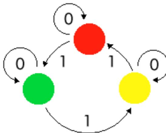
Figure 1.13 A State diagram of traffic signal sequence (a single light)
