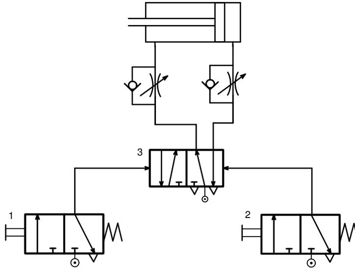
Figure 2.25 Memory function of double acting cylinder control
