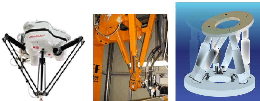
Figure 4.11 Delta type (left); triceps type (mid) Hexapod type (right) **Parallel Robots**
