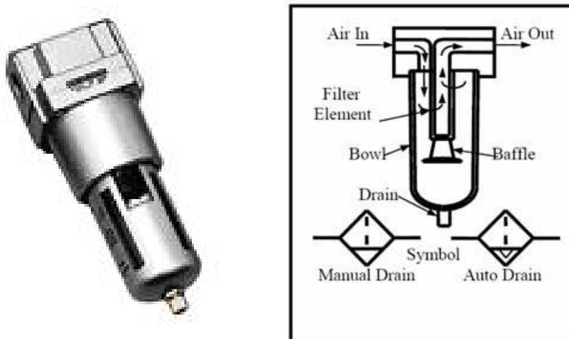
Figure 2.3 Typical structure and symbol of a Filter with Drain
