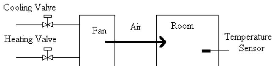
Figure 1.26 Block diagram of temperature feedback control system
