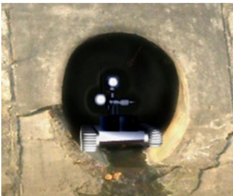
Figure 3.1 A typical pipe inspection robot
