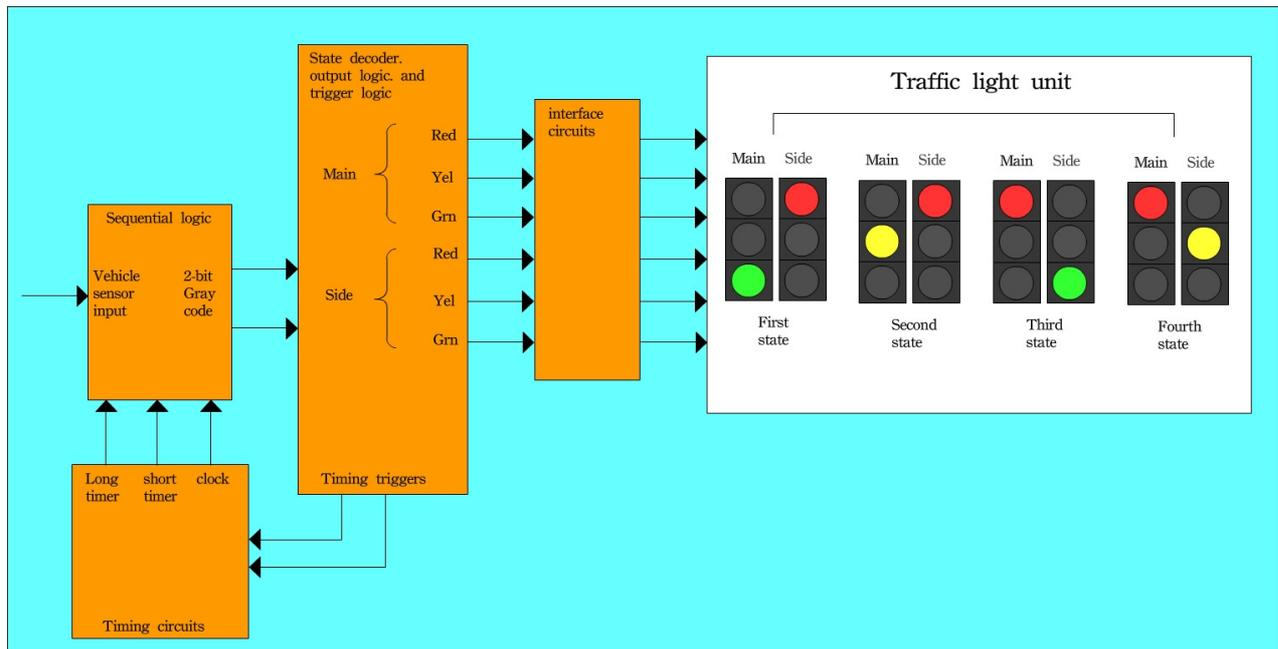
Figure 1.14 A Block Diagram of Typical Traffic Control system
