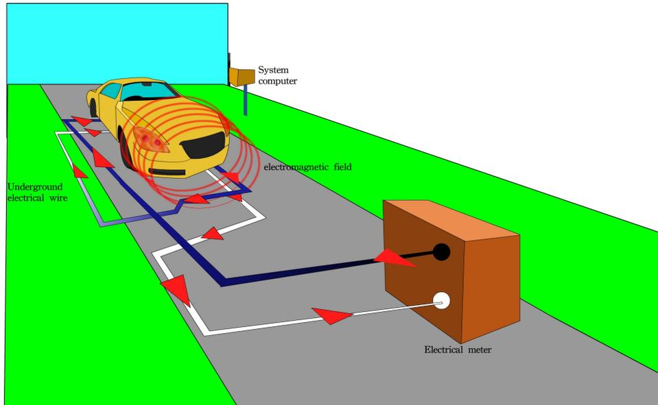
Figure 1.15 A diagram of Induction loop traffic sensor.
