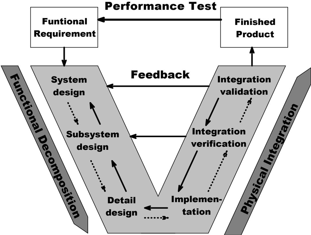
Figure 1.7 Vee Model of System and Sub-system approach
