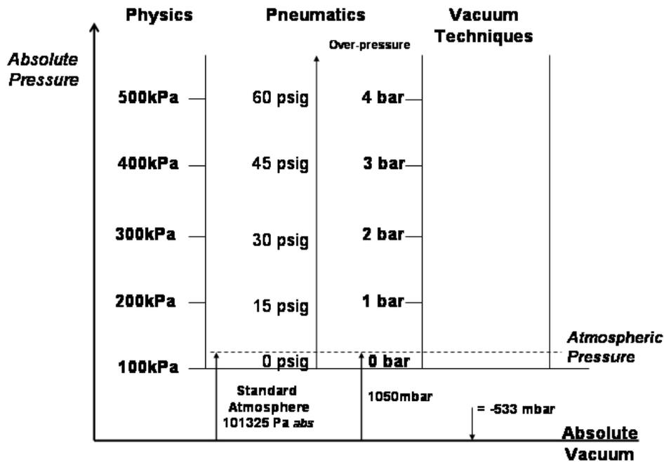
Figure 2.1 The various systems of pressure notation
