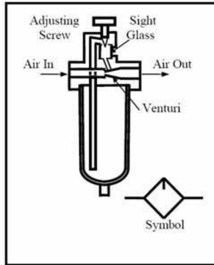
Structure and symbol of a Lubricator
